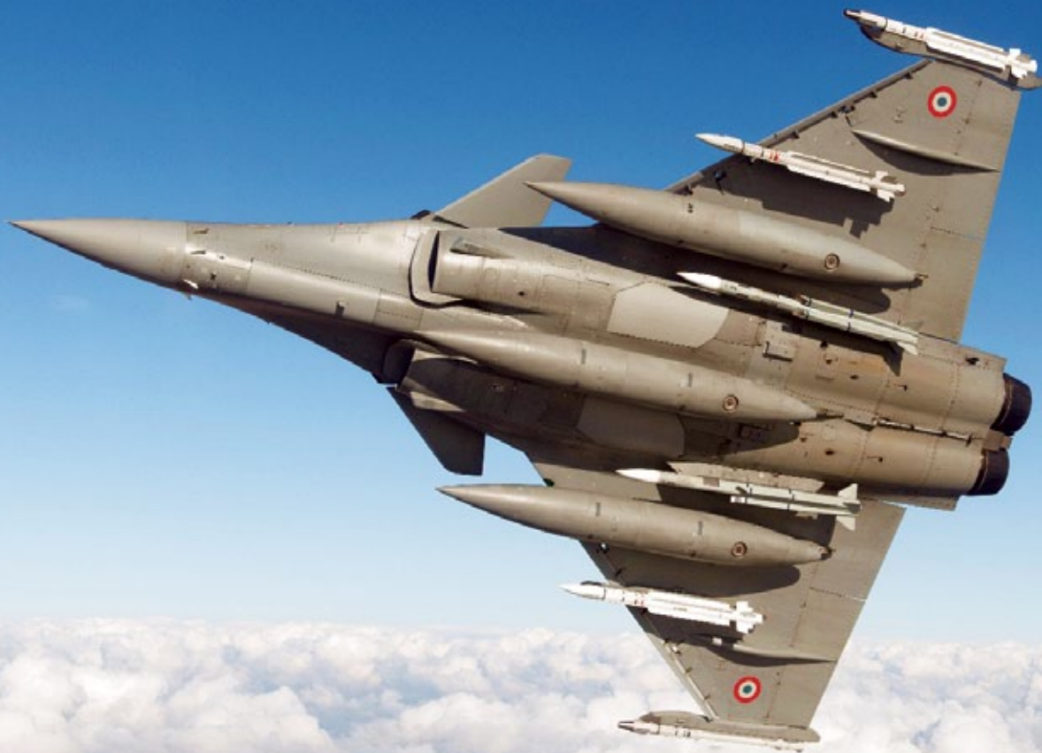
French Air Force Rafale (in this photo) but soon to be with the IAF as an operator of the type, is seen here with two MBDA Meteor's and four MICA AAMs. (photo: Dassault)
