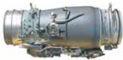
The Adour engine powers both the Jaguar and Hawk with the IAF
