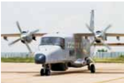
A pair of Honeywell TPE331-5s on an Indian Navy Dornier 228 (photo: Angad Singh)
