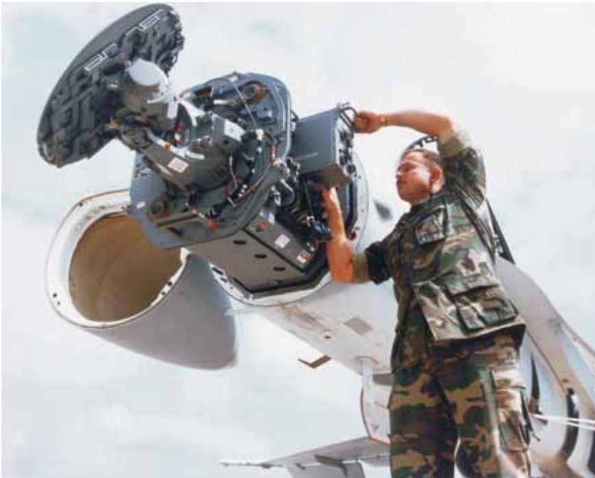
Mechanically-steered antenna on a F/A-18C Hornet undergoing maintenance
