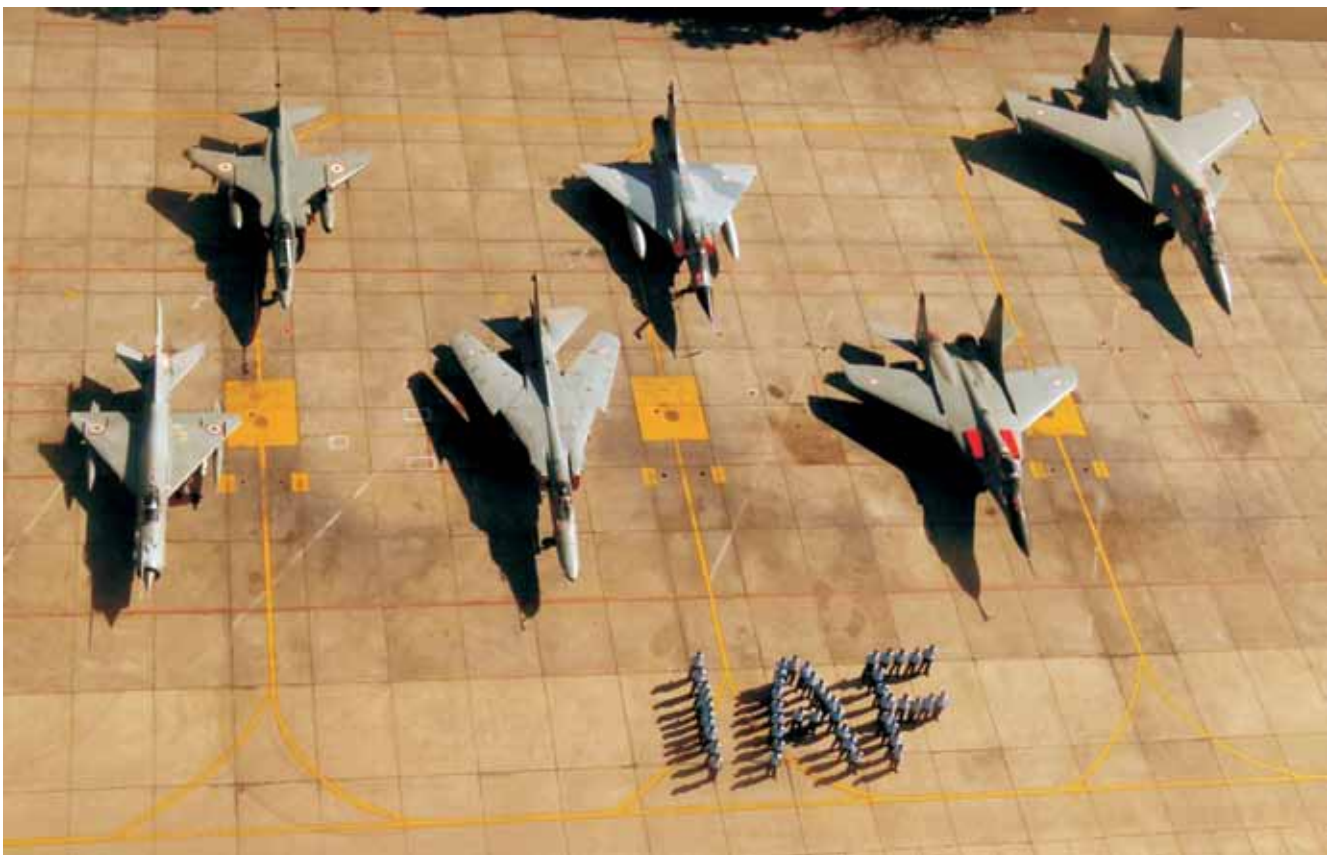
Mix of combat aircraft types operated by the IAF today : MiG-21, Jaguar, MiG-27, Mirage 2000, MiG-29 and Su-30MKI : these are to be supplanted by the LCA, MMRCA, AMCA FGFA in the next decades
