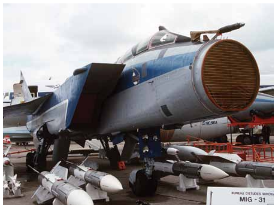
The Tikhomirov BRLS-8B 'Zaslav' was the first PESA to be installed in an aircraft (the MiG-31 interceptor)
