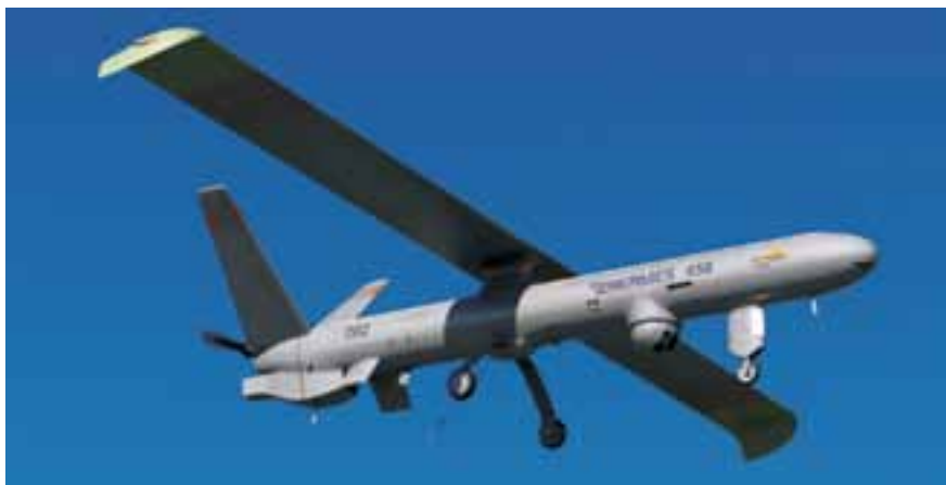
Hermes 450 seen in flight with an electro-optical surveillance payload
