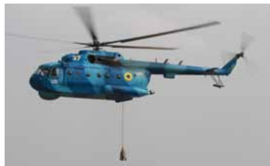
One of the Mi-14 helicopters shows its dipping sonar, used to detect and track submarines
