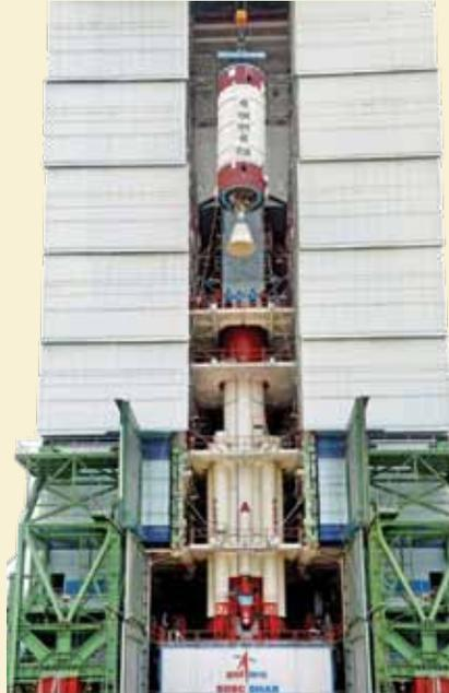
*Hoisting of PSLV-C38 second stage during vehicle integration*
