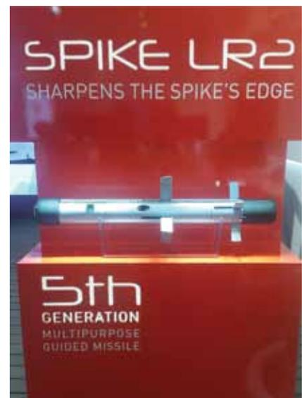
Spike LR II has a range of 5.5 km when fired from ground launchers (an increase of more than 35% beyond the 4 km range of the original Spike LR) and up to 10 km when fired from a helicopter (using alternative option of RF Data link). The Spike LR II has a modern electro-optical seeker which includes a high quality un-cooled IR sensor and an advanced high definition colour day sensor. The new seeker includes capabilities of a smart target tracker with AI features.
