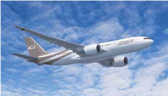
Airbus Corporate Jets has launched a private jet version of its new A330neo, which combines new-generation engines and aerodynamic and other improvements to deliver “even more comfort, efficiency and true non-stop to the world” range. The ACJ330neo will fly 25 passengers 9,400 nm/17,400 km or 20 hours, for non-stop air services from Europe to Australia.
