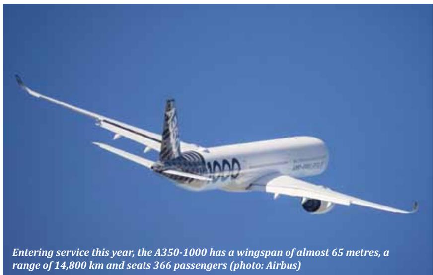
*Entering service this year, the A350-1000 has a wingspan of almost 65 metres, a range of 14,800 km and seats 366 passengers (photo: Airbus)*
