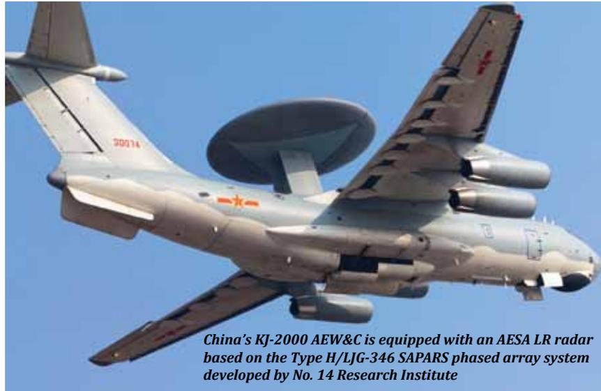
**China's KJ-2000 AEW&C is equipped with an AESA LR radar based on the Type H/LJG-346 SAPARS phased array system developed by No. 14 Research Institute**
