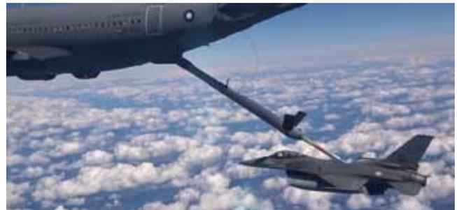
Airbus Defence and Space have demonstrated automatic air-to-air refuelling (AAR) contacts with a fighter aircraft from a tanker's refuelling boom the first time that this has been done. The Airbus' A310 MRTT development aircraft performed six automatic contacts with a F-16 of the Portuguese Air Force in a demonstration of a technique which the company believes holds great promise for enhancing in-service AAR operations.
