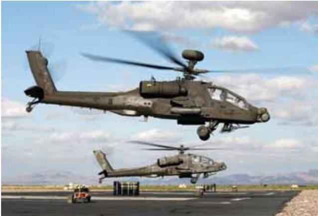
The Republic of Singapore Air Force has embarked on an upgrade programme for its AH-64D Apache fleet. The attack helicopters have been equipped with “new mission systems to enhance the helicopter’s survivability and improve its mission capability.” The upgrade includes integrating the Helicopter Integrated Electronic Warfare System (HIEWS) and SATCOM and the programme is expected to be completed “over the next few years.”
