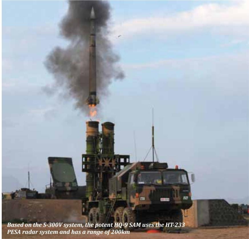
Based on the S-300V system, the potent HQ-9 SAM uses the HT-233 PESA radar system and has a range of 200km
