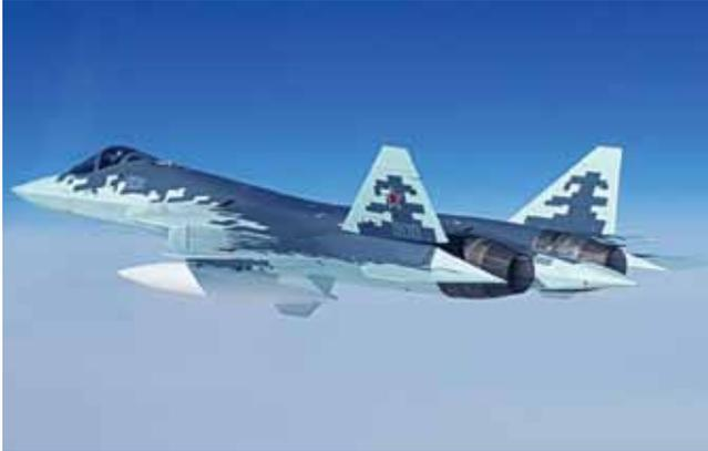
The latest prototype of Sukhoi's PAK FA fifth-generation fighter project, T-50-9, reportedly made its first flight at Komsomolsk-on-Amur on 24 April. Aircraft '509' differs from its predecessors in having a 'pixelated' camouflage scheme, the aircraft also undergoing trials with new underwing drop tanks.
