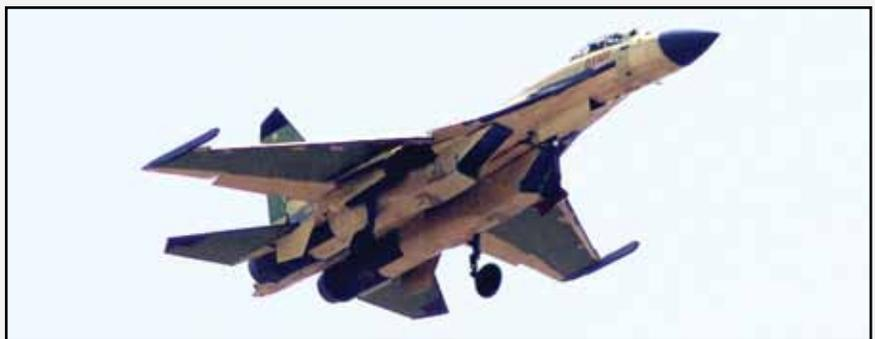
*The J-11D prototype (D1101) under testing. The J-11D will be the most advanced version of the J-11, rivalling the Russian Su-35 in many areas. Note the flattened Radome*
