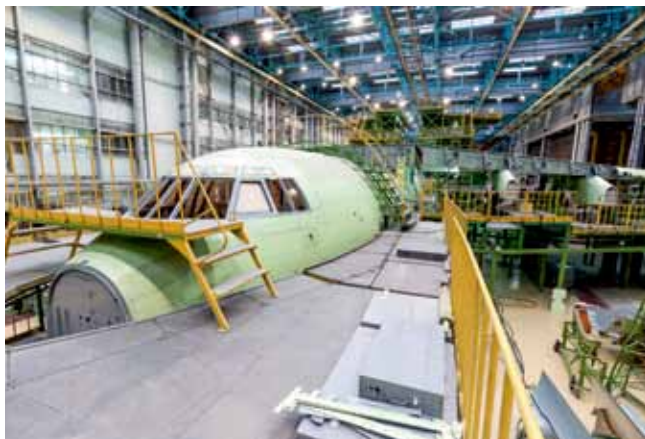
Il-78M-90A wing-fuselage mating at Aviastar-SP, Ulyanovsk (photo: Angad Singh)
