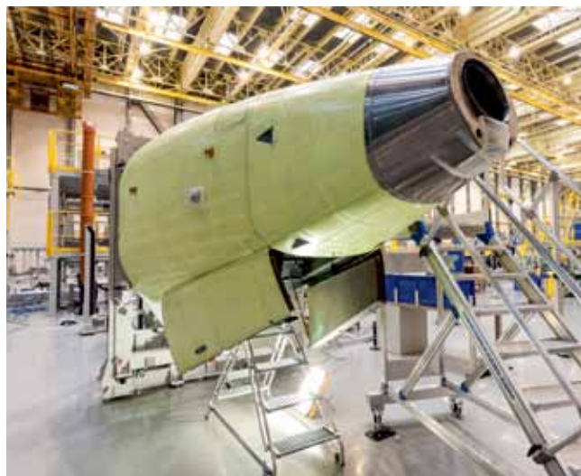
MC-21 APU housing and tailcone under construction at Aviastar-SP in Ulyanovsk (photo: Angad Singh)
