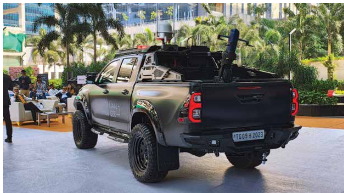
Rear profile of Ranger, with Zombee Interceptor and roof mounted drone detection system.
