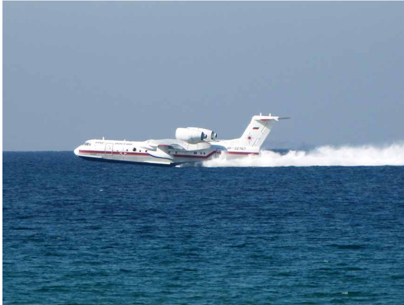
Russia's Beriev Be-200 filling water tanks in the Mediterranean Sea while in operation against the 2010 Mount Carmel forest fire in Israel (Photo: Wikipedia)
