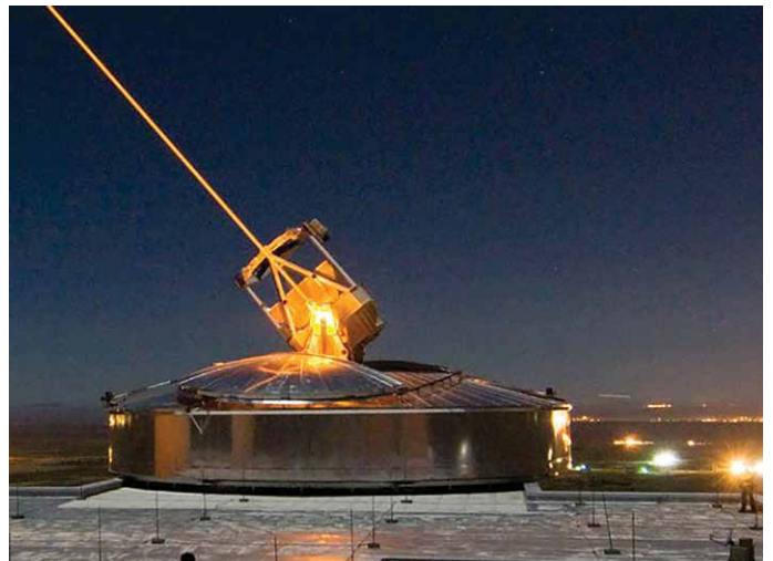
The Sodium Guidestar at the US Air Force Research Laboratory Directed Energy Directorate's Starfire Optical Range. Researchers with AFRL use the Guidestar laser for real time, high fidelity tracking and imaging of satellites too faint for conventional adaptive optical imaging systems. The SOR's adaptive optics telescope is the second largest telescope in the Department of Defence. (Photo: AFRL)
