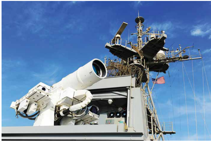
The US Navy's Laser Weapons System (LaWS) aboard the USS Ponce in the Persian Gulf (Photo: USN)
