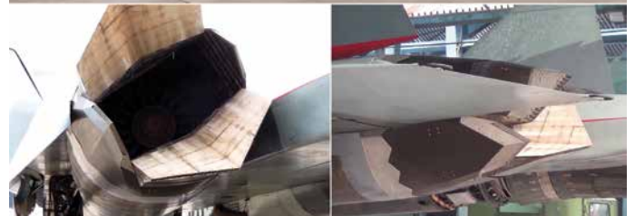
New flat nozzle of the Su-57 (Source: X/Russia)
