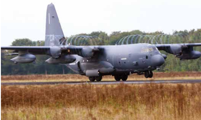
This HC-130J 'Combat King II' is rarely seen in Europe. It is the only dedicated fixed-wing personnel recovery platform in the US Air Force inventory of which there are some three dozen operational. The moist air makes for the 'corkscrew' vapour trails.
