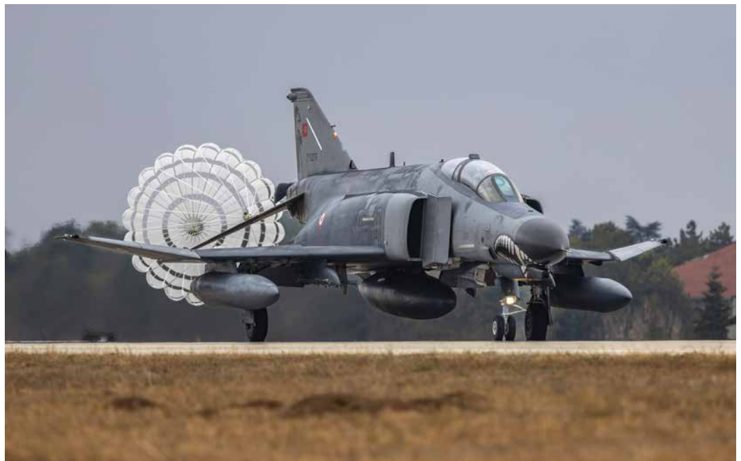
F-4E with typical dragchute.
