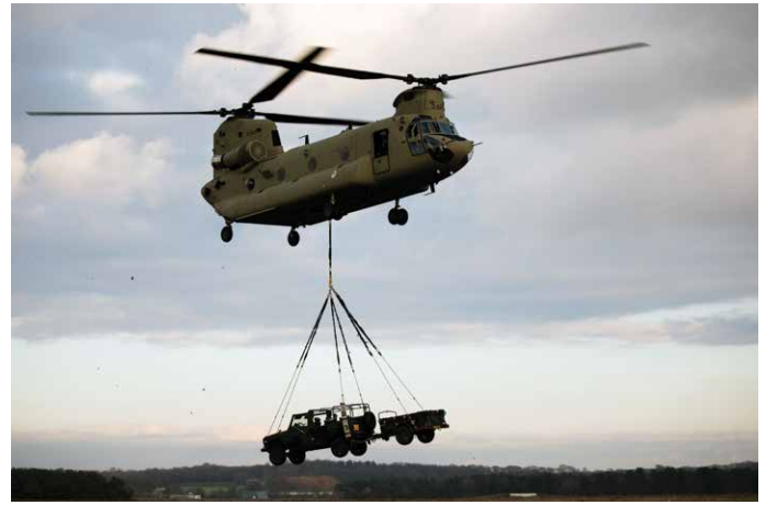
Mercedes-Benz G280 CDI off-road vehicle with trailer arriving by Chinook at the landing zone.
