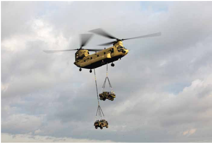
A Chinook approaches her landing zone while transporting two Airmobile Special Vehicle.
