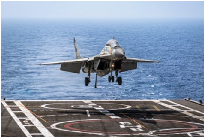
IN831 approaches the flight deck of INS Vikramaditya on its way to a perfect middle-wire trap...
