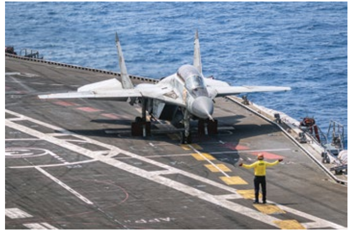
A MiG-29K is directed onto the hydraulic restraining gear on INS Vikramaditya’s flight deck to make ready for launch.
