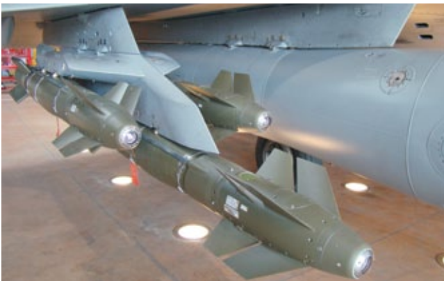
For precision strike missions, the Rafale is fitted with six Sagem AASM Hammer INS-GPS-IR guided weapons.
