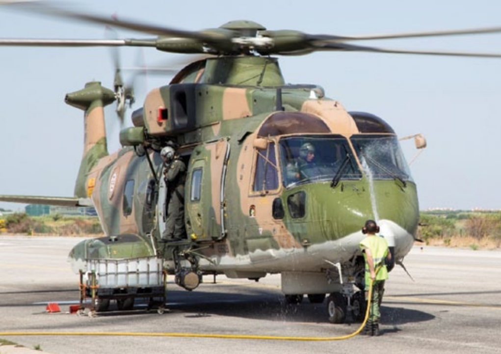
Merlins are washed after every a mission over the sea, to prevent corrosion
