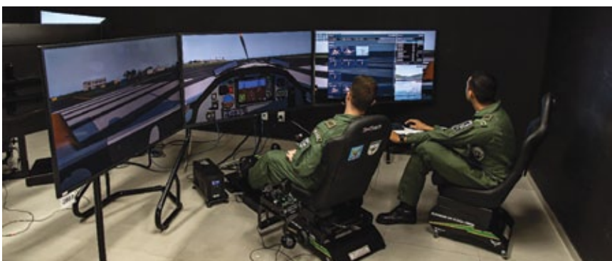
The T-2000 simulator uses 3 screens and can be configured as the T-25 and the T-27. It's an ideal system for the cadets to get initial and additional training.
