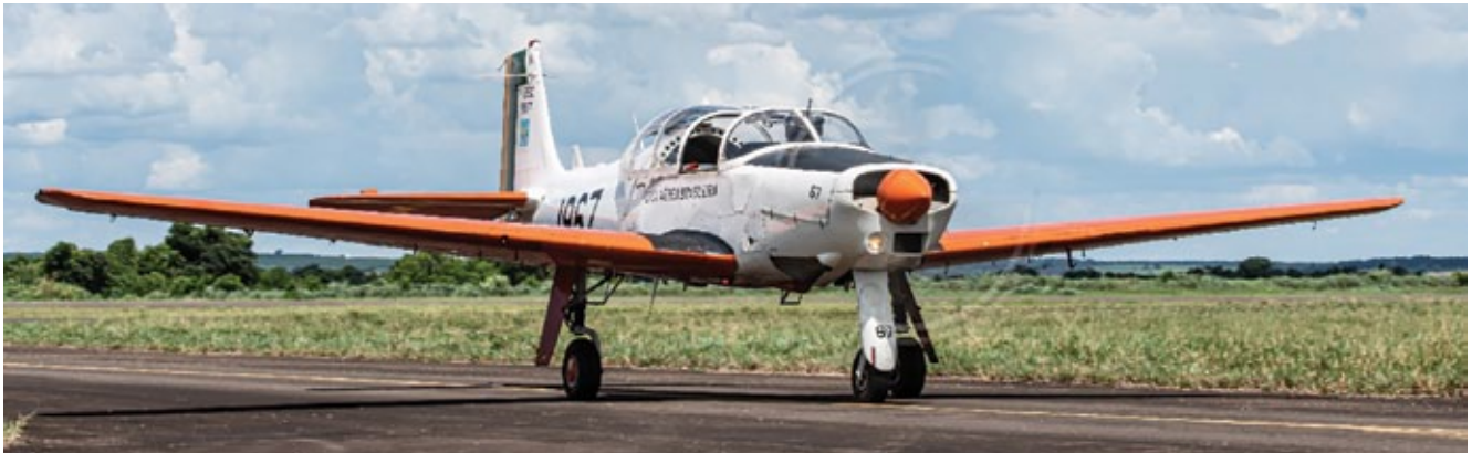
The AFA uses the T-25A and T-25C. The main difference is the T-25C has different avionics, making it more suitable for navigation training flights.
