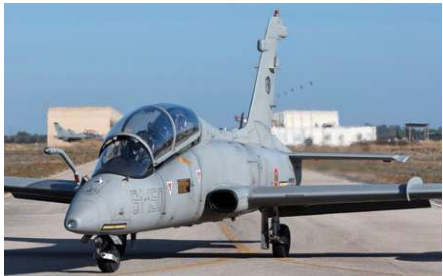
Frontal view of MB-339CD, the upgraded version of MB-339A. Note the different nose and the in-flight refueling probe
