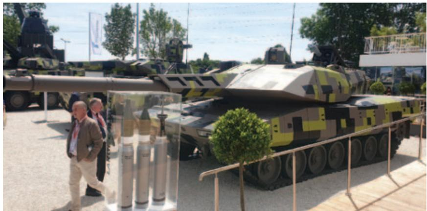
gun and a fully automatic ammunition handling system. The autoloader holds 20 ready rounds. Compared to current 120 mm systems, the FGS delivers over fifty percent greater effectiveness at significantly longer ranges of engagement. The FGS can fire kinetic energy (KE) rounds as well as programmable airburst ammunition and corresponding practice rounds.
