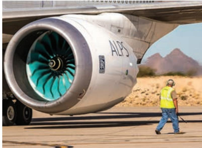
a variable pitch fan system, is based on technology that could be ready for service from 2025 and will offer at least 25 per cent less fuel and CO<sub>2</sub> emissions against the same baseline. CTi technology delivers lighter fan blades while retaining aerodynamic performance.
