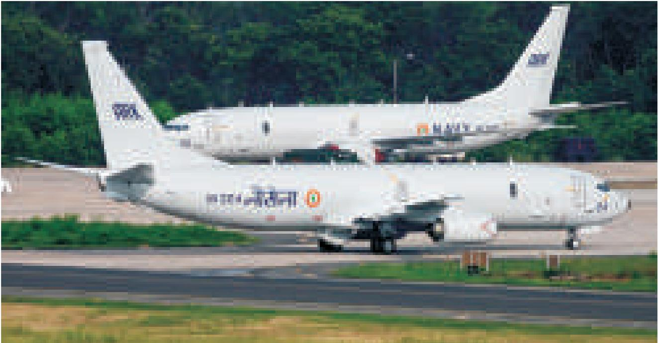
*Radome for the aft radar and the slender MAD boom can be seen in this image as IN324 taxis back to the apron*
