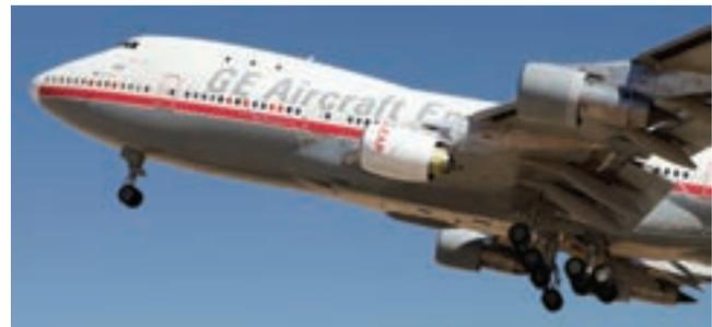
The engine “behaved well and completed multiple aeromechanical test points at various altitudes during the nearly three-hour first flight.” Over several weeks, the engine will complete a comprehensive test schedule that will gauge engine operability, stall margin, performance, and acoustics. The LEAP-1A/-1C variants are on track for engine certification in 2015.
