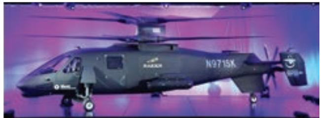
rigid X2 rotor coaxial design, the S-97 Raider helicopter features next-generation technologies in a multi-mission configuration (armed aerial scout or light assault), capable of carrying six troops and external weapons. Sikorsky will offer the Raider aircraft as replacement for the US Army's OH-58D Kiowa Warrior helicopter fleet based on the Army's future operational and financial priorities, and for the special operations platform.
