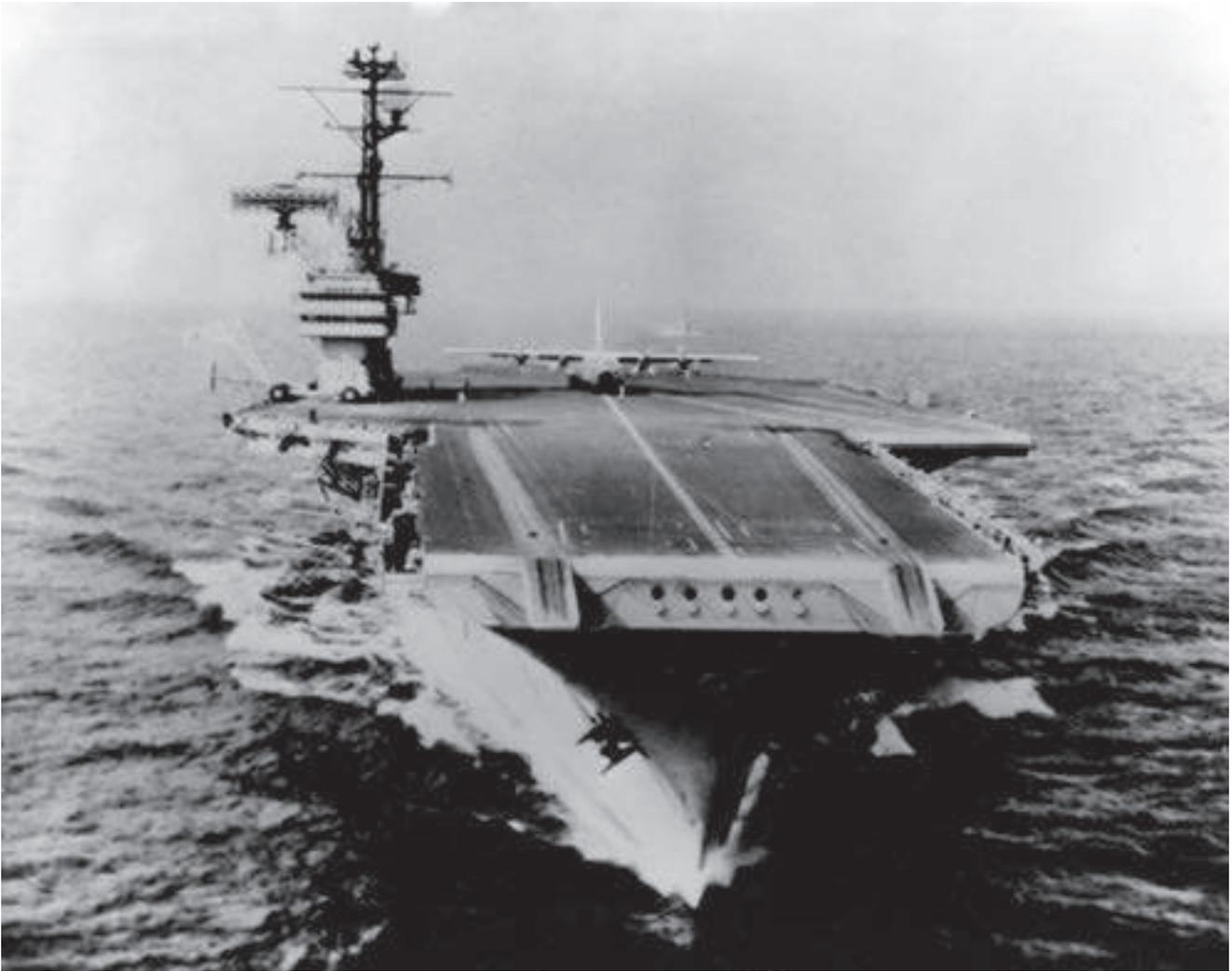
*The KC-130 weighed 85,000 pounds on the first landing. Thereafter, landings were made in progression up to a gross weight of 121,000 pounds. One landing at a weight of 109,000 pounds required 495 feet to stop and that was in a heavy squall. On the last takeoffs, the crew didn't even back up—they simply took off from the point on the deck where the aircraft stopped!*
