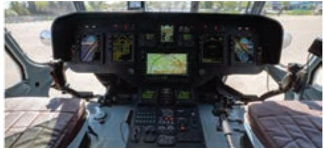
satellite system displays, mapping, flight-plan navigation systems (VOR/ILS), meteorological information and automated obstacle warning systems.
