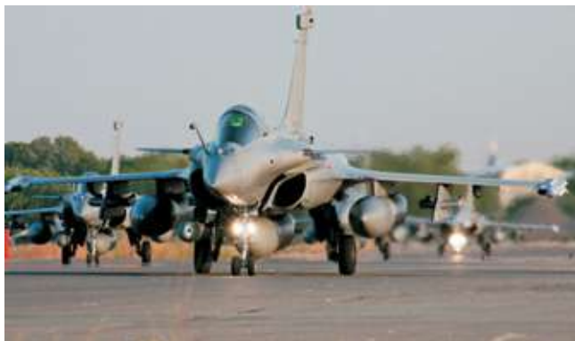
A quartet of Rafales seen at N'Djema following the strike on Gao (note empty bomb racks)
