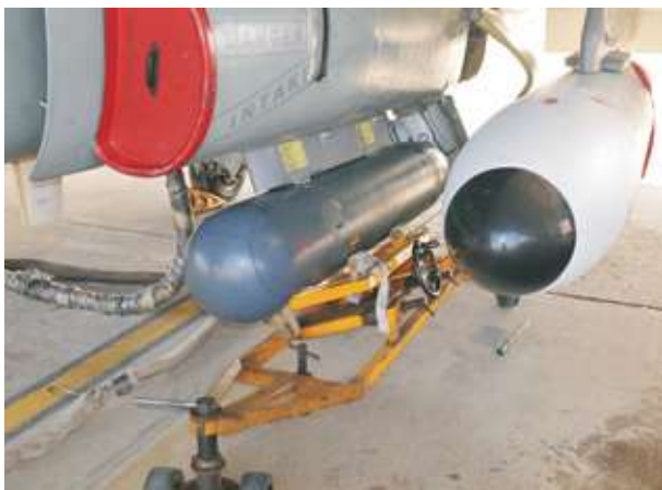
Tejas LCA with Litening pod and fuel droptank.
