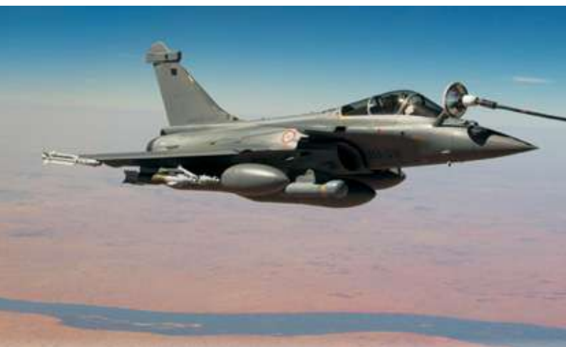
Rafale refuelling over Africa. MBDA MICA on wingtips, GBU-12 LGBs on bomb racks, and Thales Damocles pod on the starboard fuselage pylon.
