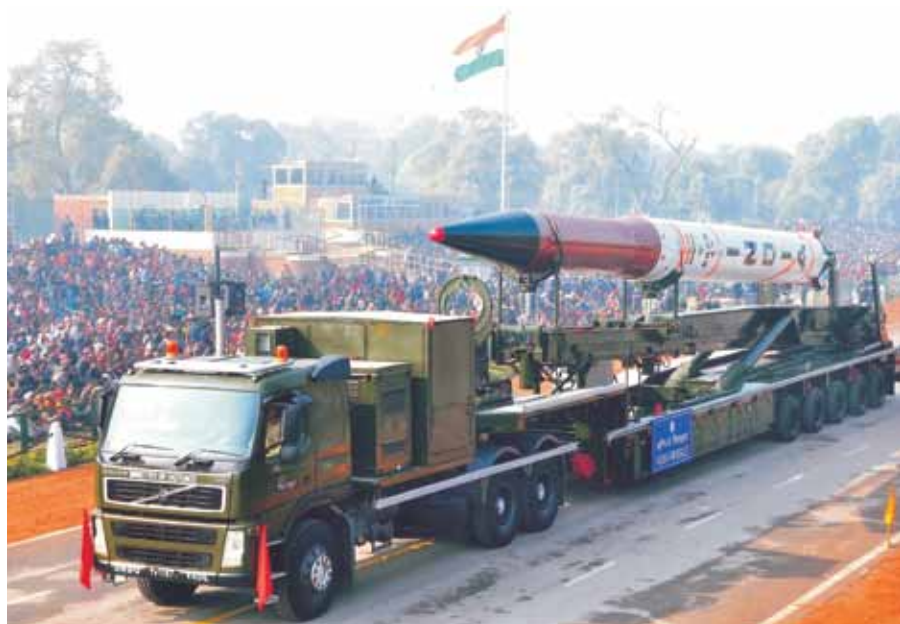
Agni-4, the two-stage surface-to-surface IRBM.
