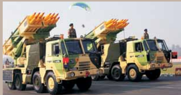
The Pinaka unguided rocket system and area weapon system loaded on a multi barrel launcher.
