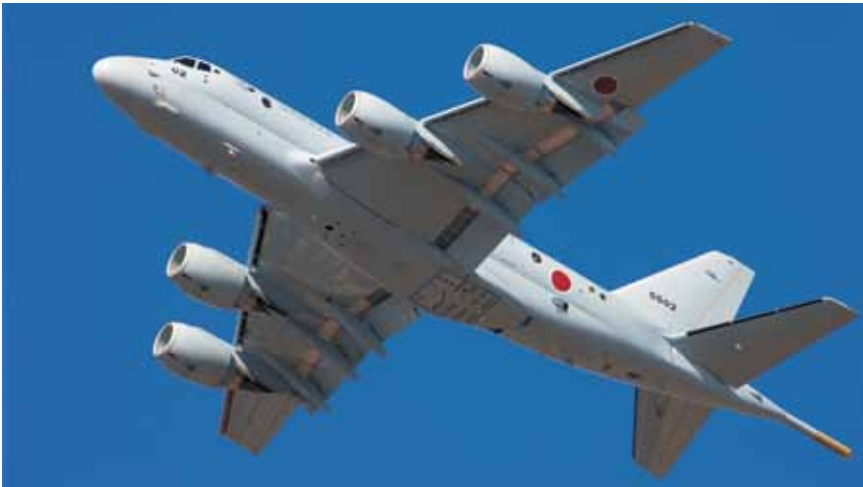
Resurgence of Japan's aerospace industry : the Kawasaki P-1 long range maritime patrol aircraft, designed to replace the venerable Lockheed P-3C Orion with the JMSDF.
