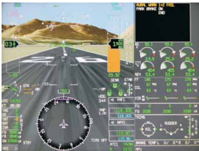
EASy II cockpit display with synthetic vision in CAE Dassault Falcon 900EX full-flight simulator at Morristown, New Jersey.
