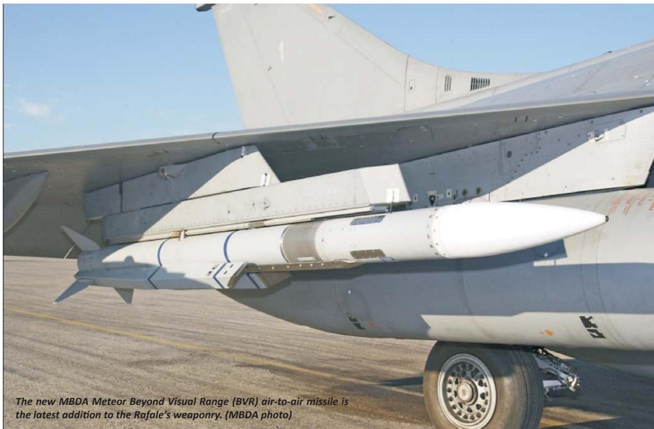
*The new MBDA Meteor Beyond Visual Range (BVR) air-to-air missile is the latest addition to the Rafale's weaponry. (MBDA photo)*
