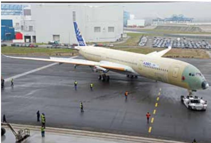
Airbus' first A350 XWB moved to the next phase of ground testing with its transfer from the final assembly line to the Clément Ader area 'Station 18' in Toulouse, which is primarily dedicated to fuel, pressure and radio navigability evaluations.
