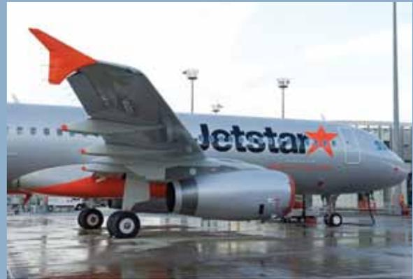
The A320neo (new engine option) is the latest of many product upgrades as Airbus continues to invest around 300 million euros a year on the A320 Family. These new A319, A320 and A321 models were announced in December 2010 and feature new engines (the PurePower PW1100G from Pratt and Whitney or the LEAP-1A from CFM) and large wingtip devices known as Sharklets. Together they result in a 15% fuel burn reduction, corresponding to an annual CO<sub>2</sub> reduction of 3,600 tonnes per aircraft.
