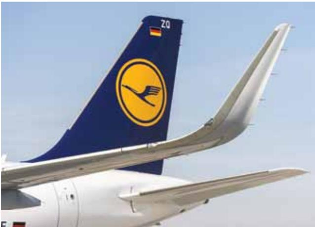
*German flag carrier Lufthansa took delivery of its first A320 outfitted with fuel-saving Sharklets on 1 March 2013, and will receive 21 more A320 Family aircraft equipped with the wingtip devices by 2015.*
