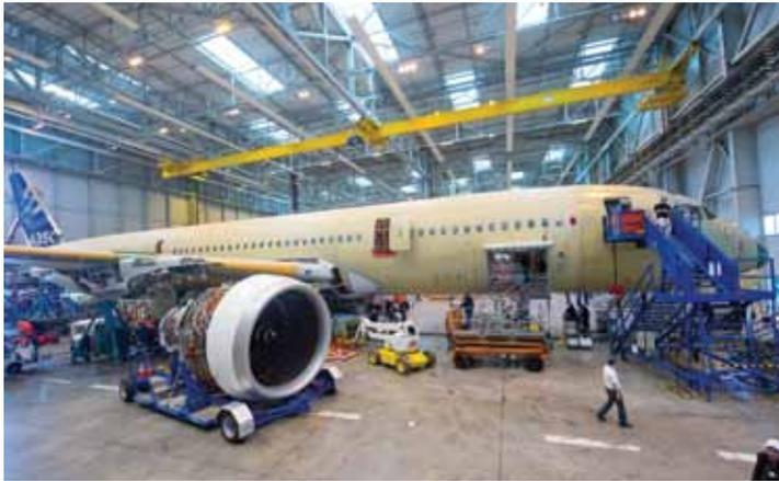
Airbus has installed its two flight-ready Rolls-Royce Trent XWB engines and the new Honeywell HGT1700 APU on the first flight-test A350 XWB (MSN001).
