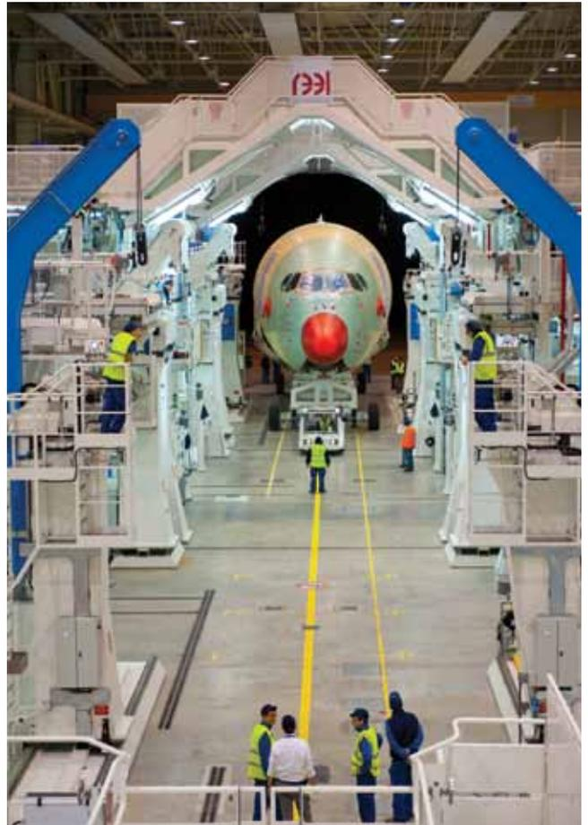
Fuselage sections for the third A350 XWB – which will be used for a wide range of evaluations in the flight test programme – were joined at the A350 XWB Final Assembly Line in Toulouse, France.
