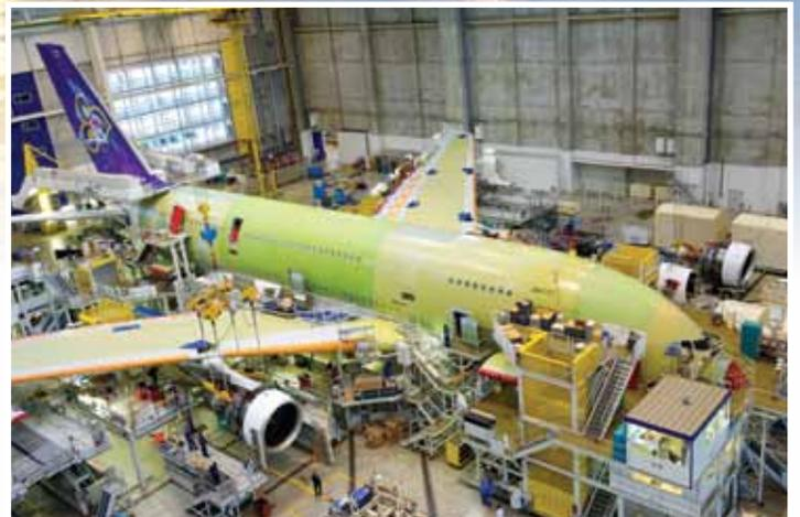
*A Rolls-Royce Trent 900 engine is mated to Thai's first A380 on the Airbus final assembly line.*
