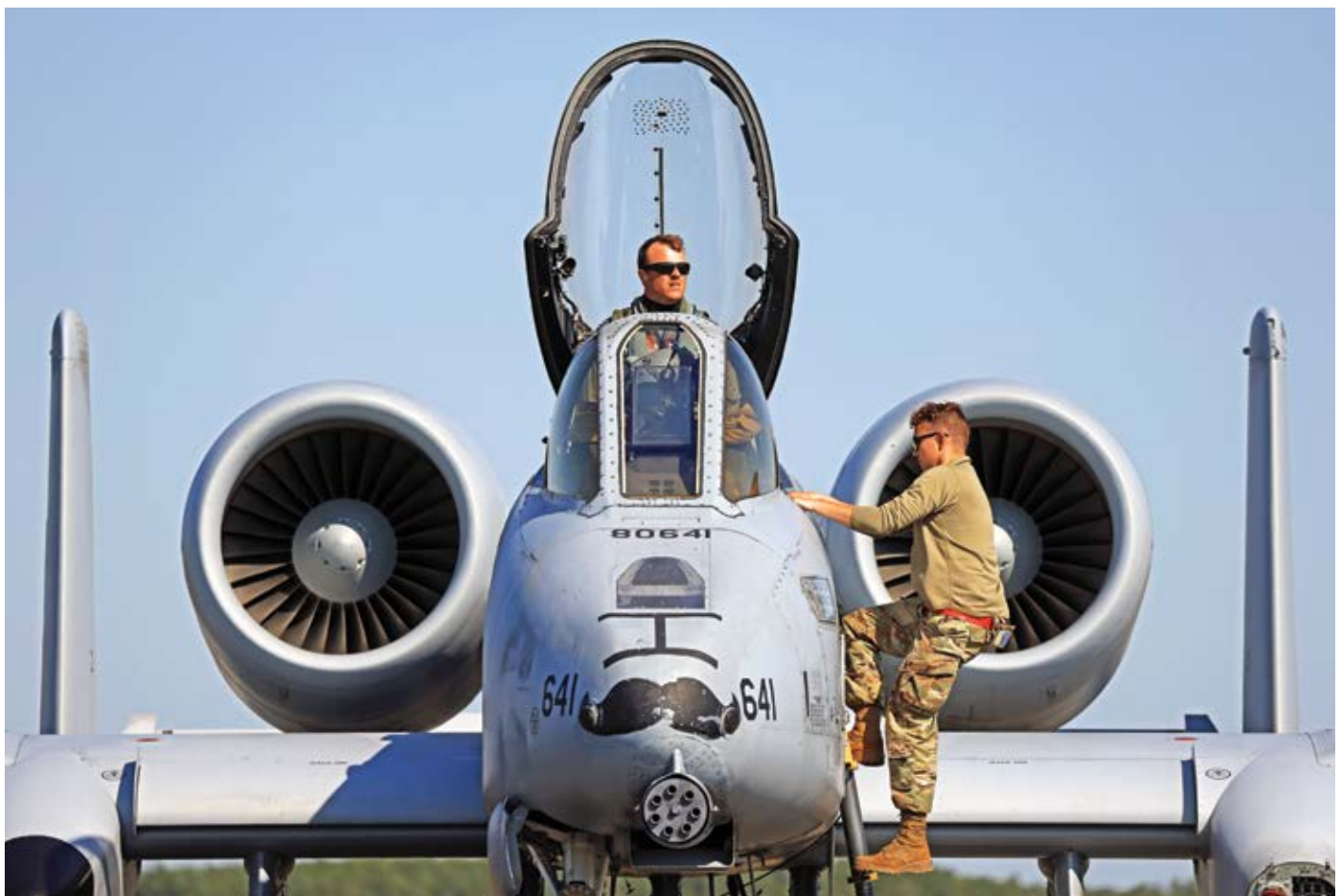
This frontal view of the A-10 Thunderbolt shows the nozzle of the huge cannon in the nose. Due to the size of this cannon, as big as a Volkswagen Beetle, the nose wheel had to be moved from the centreline of the aircraft, as can be seen here as well.
