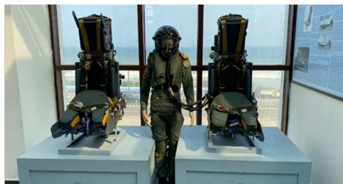
Ejection seat of the Harrier (MB MK 10 H)
