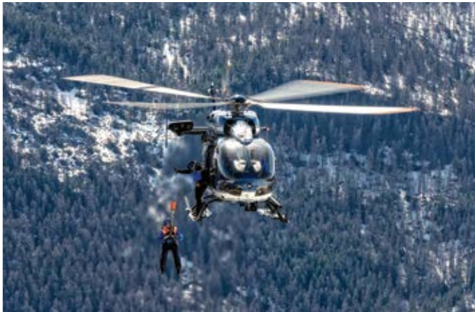
The EC145 is equipped with a hoist on the right side, here the flight engineer hoists down the mountaineer onto a drop zone.
