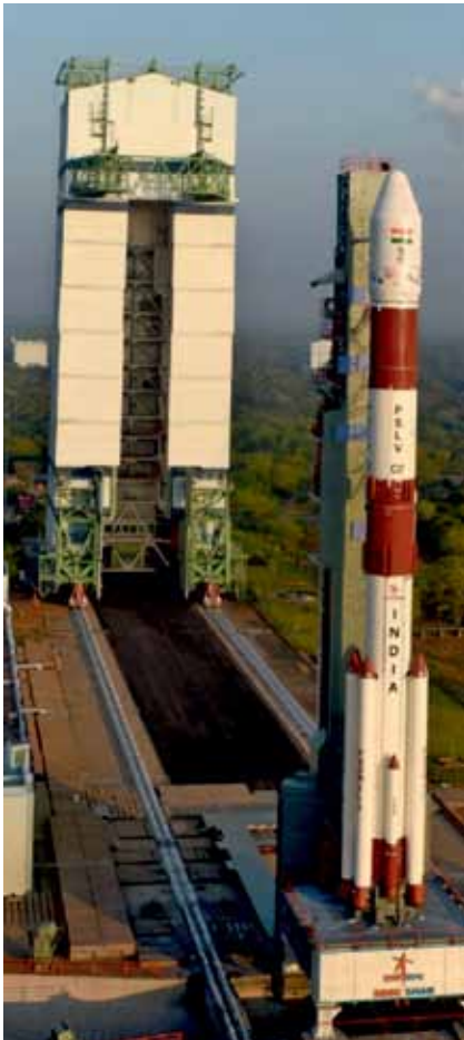
Fully integrated PSLV-C37 seen with mobile service tower
